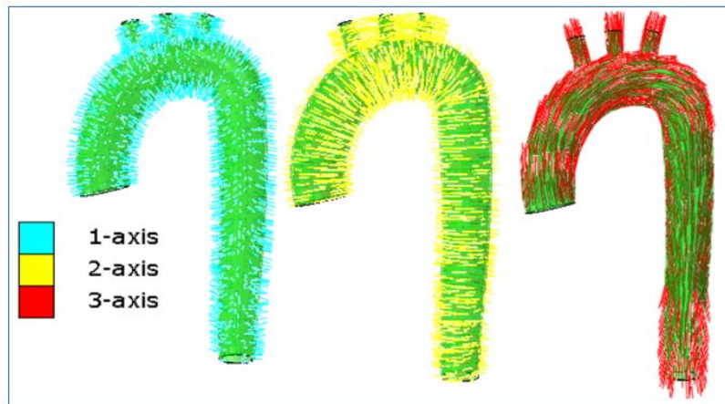
Figure 4.8: Local coordinate system for HGO material. Axis 1, 2, 3 represent radial, circumferential and longitudinal/axial directions, respectively.
